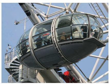
not usually stop to take on passengers; the rotation rate is slow enough to allow passengers to walk on and off the moving capsules at ground level. It is, however, stopped to allow disabled or elderly passengers time to embark and disembark safely.
